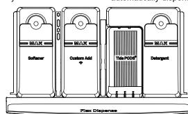
HE detergent should be added to the far right compartment. Follow the detergent manufacturer's recommendations for the correct amount of detergent, based on load size, taking care to add detergent to the right compartment. Do not overfill or dilute detergent as this can result in additive being dispensed prematurely in the wash cycle. Your option selections will determine when detergent is automatically dispensed at its optimal time in the wash cycle.
