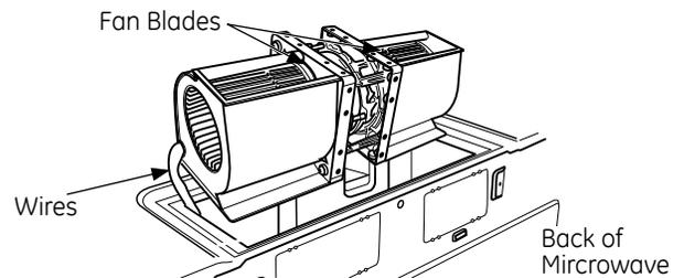
**Note:** Make sure the wires remain routed through the openings in the motor frame. To avoid damage to the fan motor wiring, insert motor carefully such that the fan motor wiring does not contact the microwave power cord bracket.
