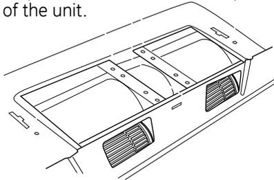
**Note:** Make sure the wires remain routed through the openings in the motor frame. To avoid damage to the fan motor wiring, insert motor carefully such that the fan motor wiring does not contact the microwave power cord bracket.
