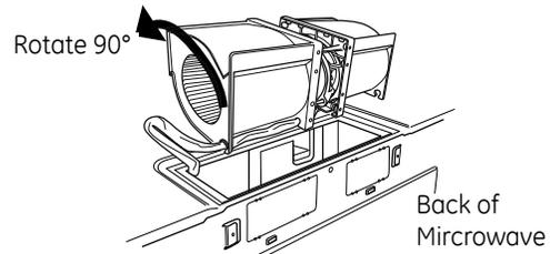
**Note:** Make sure the wires remain routed through the openings in the motor frame. To avoid damage to the fan motor wiring, insert motor carefully such that the fan motor wiring does not contact the microwave power cord bracket.
