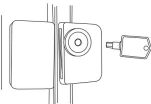
The key for the spring-loaded lock is automatically ejected—key will not remain in lock in either the open or closed position.
