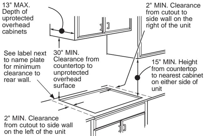
If a 30" clearance between the cooking surface and overhead combustible materials or metal cabinets cannot be maintained, a minimum clearance of 24" is required and the underside of the cabinets above the cooktop must be protected with not less than 1/4" insulating millboard covered with sheet metal not less than 0.0122" thick.
