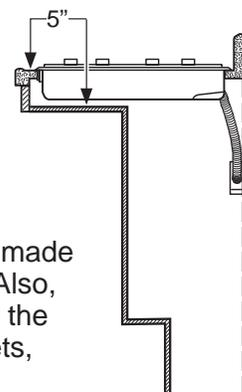
NOTE: The enclosure must be made of at least 1/4" wood material. Also, an access panel is required for the junction box, hold-down brackets, and service.
