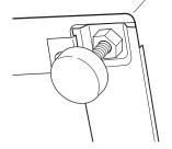
**NOTE:** To minimize vibration, the locking nuts must be tight.
