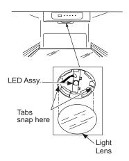
The LED light is located behind a light lens in the celling of the refrigerator section.
