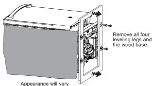
On models <u>without</u> the center bottom adjustable leveling system:
