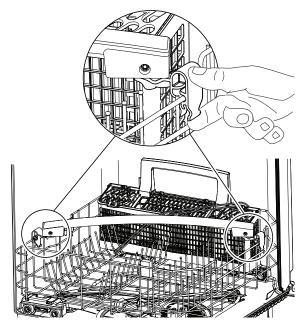
• Using the provided 1/8" Allen wrench, loosen the set screws to remove the shipping clips and discard them.
