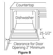
**CLEARANCES:** When installed into a corner, allow 2" min. clearance between dishwasher and adjacent cabinet, wall or other appliances. Allow 25-1/2" min. clearance from the front of the dishwasher for door opening.
