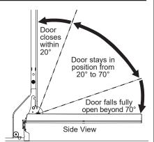
dishwasher firmly, check the door balance by opening and closing the door.
