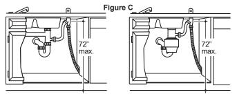
Method 2 – "High Drain Loop" with Waste Tee or Disposer
