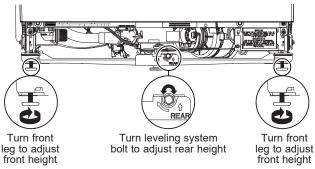
**If your model has 4 leveling feet,** adjust the level of the dishwasher by individually turning the 4 legs on the bottom of the dishwasher as shown in figure.
