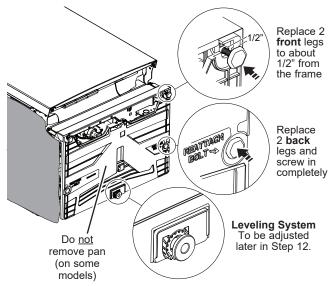
**NOTE:** Pan (on some models) should not be removed during installation.
