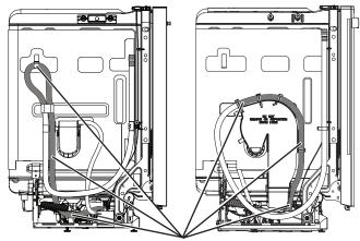
Do <u>NOT</u> detach the section of the drain hose, highlighted in **gray**, from these locations
