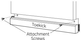
• When reinstalling the toekick, on models with a sound barrier, ensure that the bottom edge is flush with the floor. Any excess material should be tucked up behind the outer door.
