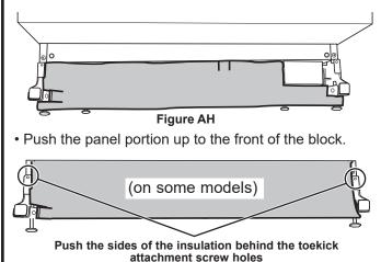
• Tuck the sides of the front panel behind the toekick attachment screw holes.
