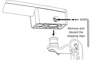
• Place the handle on the dishwasher door mounting fasteners, with the set screws on the bottom side, then tighten the set screws with the Allen wrench.
