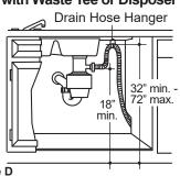
**Tip: Avoid unnecessary service call charges.** Always be sure disposer drain plug has been removed before attaching dishwasher drain hose to the disposer.
