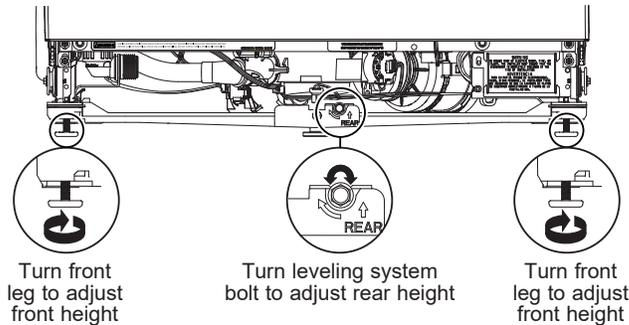
If your model has 4 leveling feet, adjust the level of the dishwasher by individually turning the 4 legs on the bottom of the dishwasher as shown in figure.
