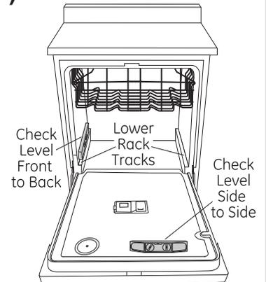
If your model has a rear leveling system, the rear height is adjusted from the front of the dishwasher along with the 2 front legs on the bottom of the dishwasher. Begin the leveling process with the front legs by individually turning the front 2 legs. Adjust the front legs first. When the front legs are adjusted to a height resulting in an appropriate gap to the upper cabinet, proceed to adjust the rear leveling system by adjusting the leveling bolt as illustrated in the figure.
