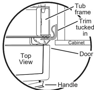
Tub trim may be trimmed if necessary to ensure proper door operation
