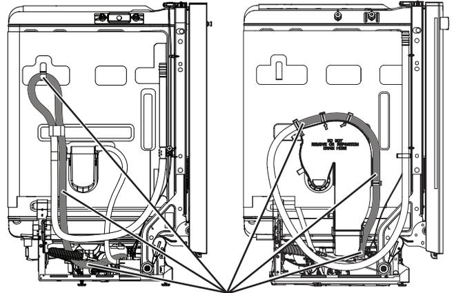
Do **NOT** detach the section of the drain hose, highlighted in **gray**, from these locations
