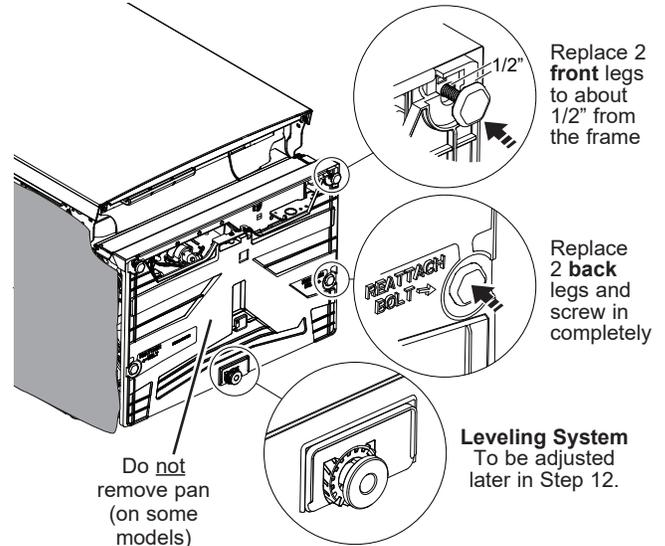
**NOTE:** Pan (on some models) should not be removed during installation.
