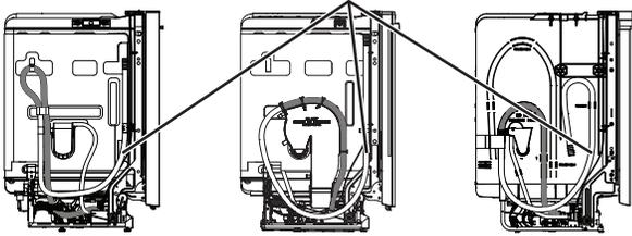
Do **NOT** detach the sections of the drain hose shown in **gray**.
