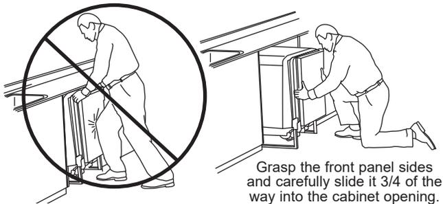
Do not push against the front door panel with knee. Damage to the door panel will occur.
