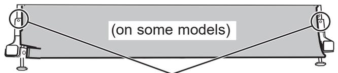
Push the sides of the insulation behind the toekick attachment screw holes
