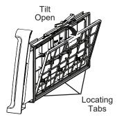
Vacuum the lint from the filter frame and inside the filter opening if you notice a change in dryer performance.
