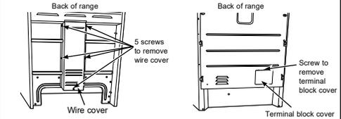
B. For power cord and 1" conduit only, remove the knockout ring (1 1/4") located on bracket directly below the terminal block. To remove the knockout, use a pair of pliers to bend the knockout ring away from the bracket and twist until ring is removed.
